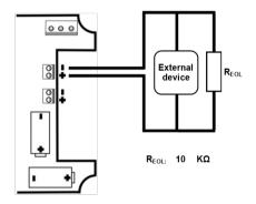
Wiring example for the relay switch output.
