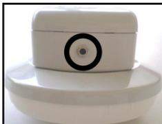
Picture 4 - the programmer's socket
