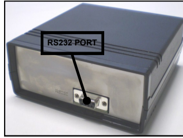
Picture 2 - Line Driver back view
